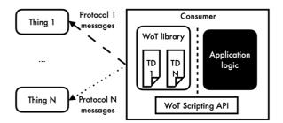
**Fig. 5** - Structure of a WoT compliant system.
