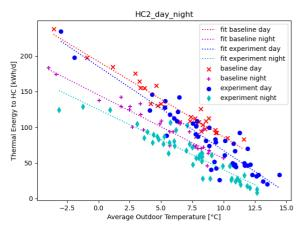
**Fig. 6** – Energy KPI with day/night split for the HC2 riser with 14 radiators over 30 days of baseline and 69 days of experiment
