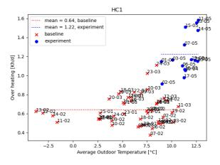
**Fig. 14** – Overheating KPI for the HC1 riser with 50 radiators over 48 days of baseline and 38 days of experiment
