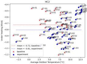
**Fig. 9** – Underheating KPI for the HC2 riser with 14 radiators over 30 days of baseline and 69 days of experiment
