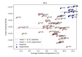
**Fig. 11** – Underheating KPI for the HC1 riser with 50 radiators over 48 days of baseline and 38 days of experiment
