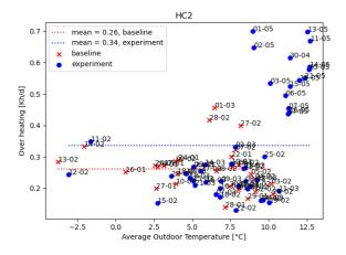
Fig. 12 – Overheating KPI for the HC2 riser with 14 radiators over 30 days of baseline and 69 days of experiment
