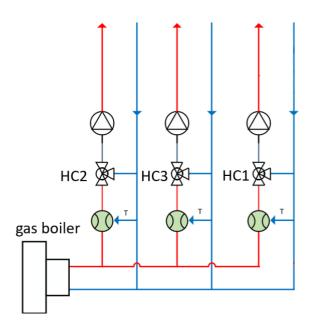
**Fig. 3** – Building heat generation and distribution layout showing three heating circuits (HC2, HC3 and HC1 from left to right).
