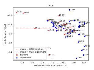
**Fig. 10** – Underheating KPI for HC3 riser with 5 radiators over 19 days of baseline and 56 days of experiment
