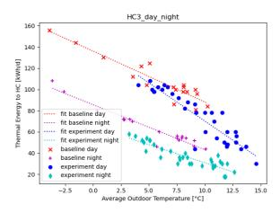
**Fig. 7** – Energy KPI with day/night split for the HC3 riser with 5 radiators over 19 days of baseline and 56 days of experiment
