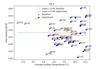
**Fig. 13** – Overheating KPI for HC3 riser with 5 radiators over 19 days of baseline and 56 days of experiment
