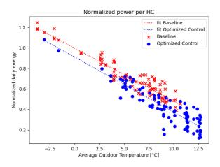
Fig. 5 – Normalized energy results for the whole building (i.e. Energy of HC1, 2 and 3 are normalized at  $0^{\circ}$ C outdoor temperature, in reference to the baseline, and aggregated)
