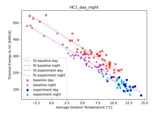
**Fig. 8** – Energy KPI with day/night split for the HC1 riser with 50 radiators over 48 days of baseline and 38 days of experiment
